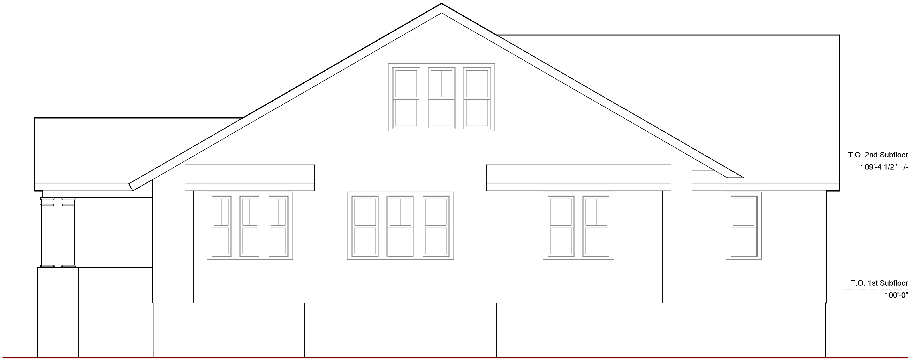
EXISTING SIDE ELEVATION
